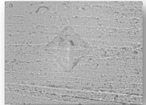
Figure 6 - Result of micro-hardness showed indentation - Reflectys
